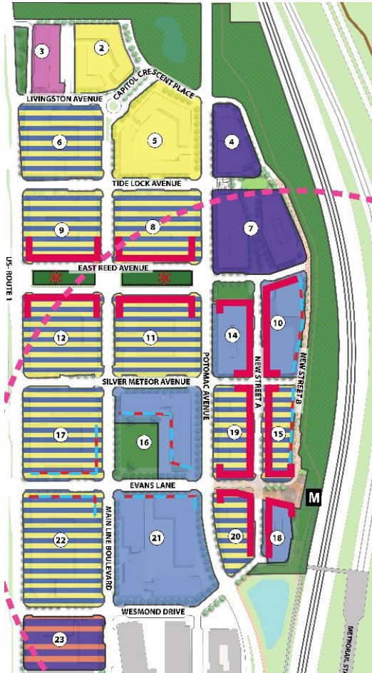
1 Figure 4.1: Land Use Plan and ¼ Mile Pedestrian Walkshed (1/2 Mile pedestrian walkshed 2 covers North Potomac Yard area) and Figure 9.1: Land Use Plan, Required and Optional Retail 3 Locations, and ¼ Mile Pedestrian Walkshed 4 5
