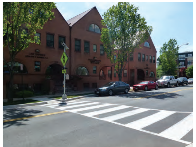
Newly installed rapid flashing beacon on Mount Vernon Avenue at Herbert Street
