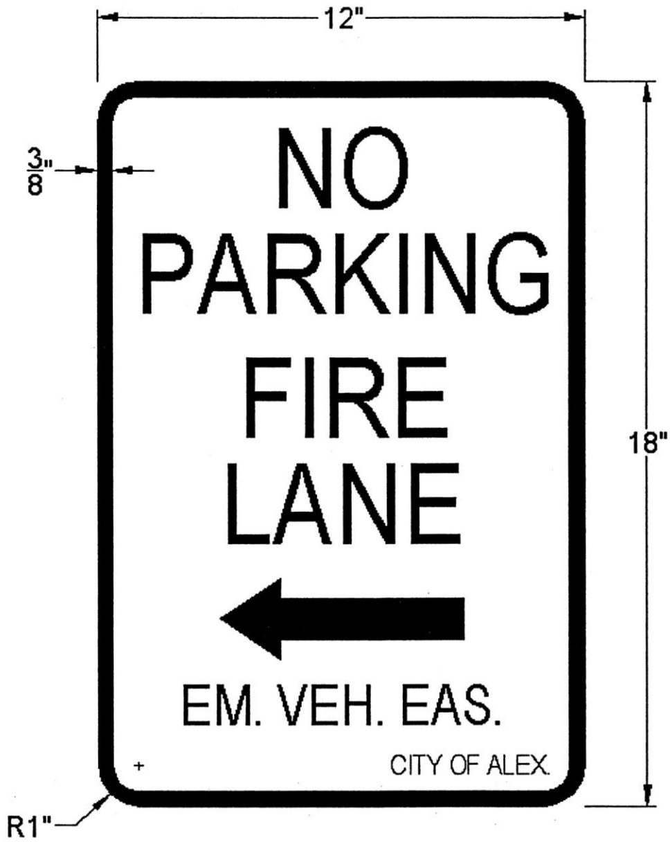
Figure-D102.1 Fire Lane Sign Left Arrow
